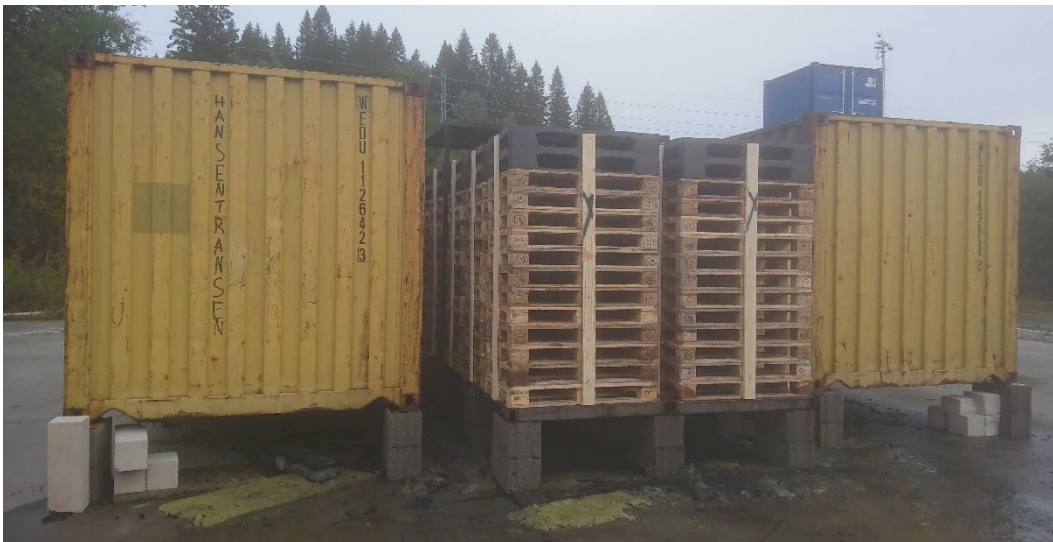
Figure 30. The main array of stacked idle wood and plastic pallets, which was partly covered by a roof, with 20 ft. cargo containers positioned parallel with and 0,5 m to the sides.
