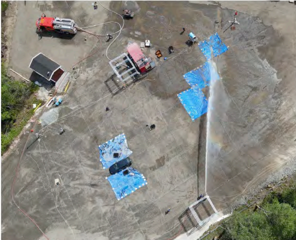
Figure 26. In one test, the snow cannon was positioned near the impact point of the maximum monitor throw length, almost opposite to the stream of water. The throw length was reduced by between 5 m and 10 m. In addition, break-up of the water stream was observed.
