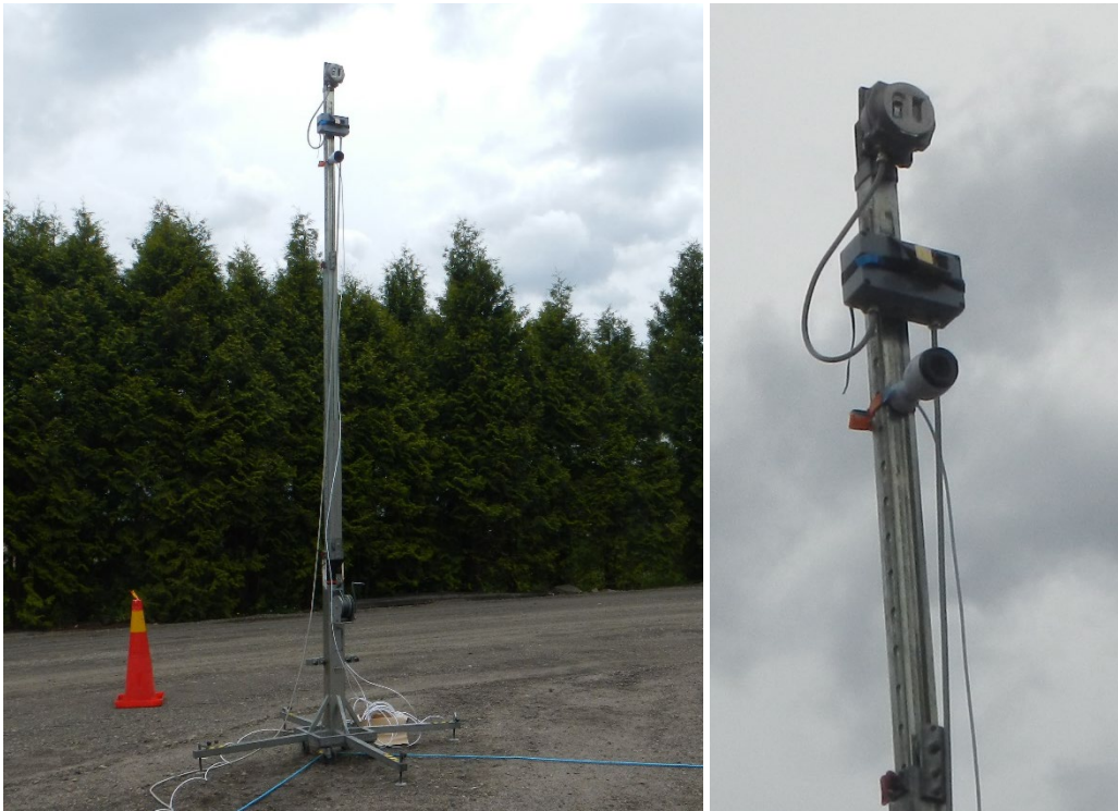
Figure 19. The support for the fire detector. The fire detector was positioned at the top and a video camera was positioned below each detector.
