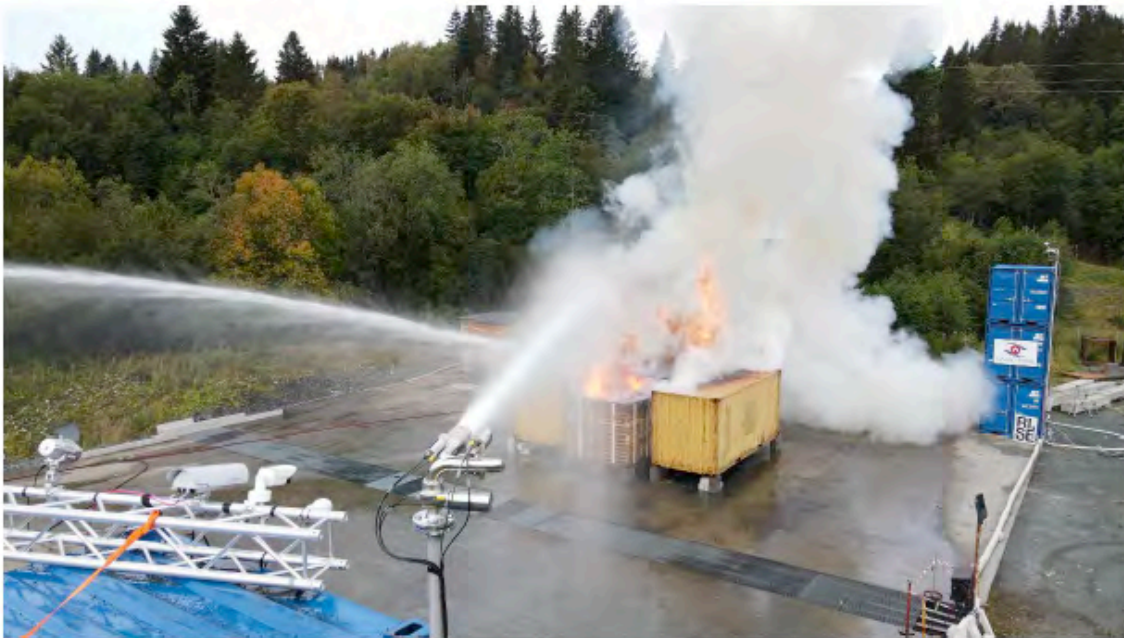
Figure 53. Test 7: The fire size a few seconds after the initial application of water from fire monitors B and C positioned at the south short-side corners of the test area.
