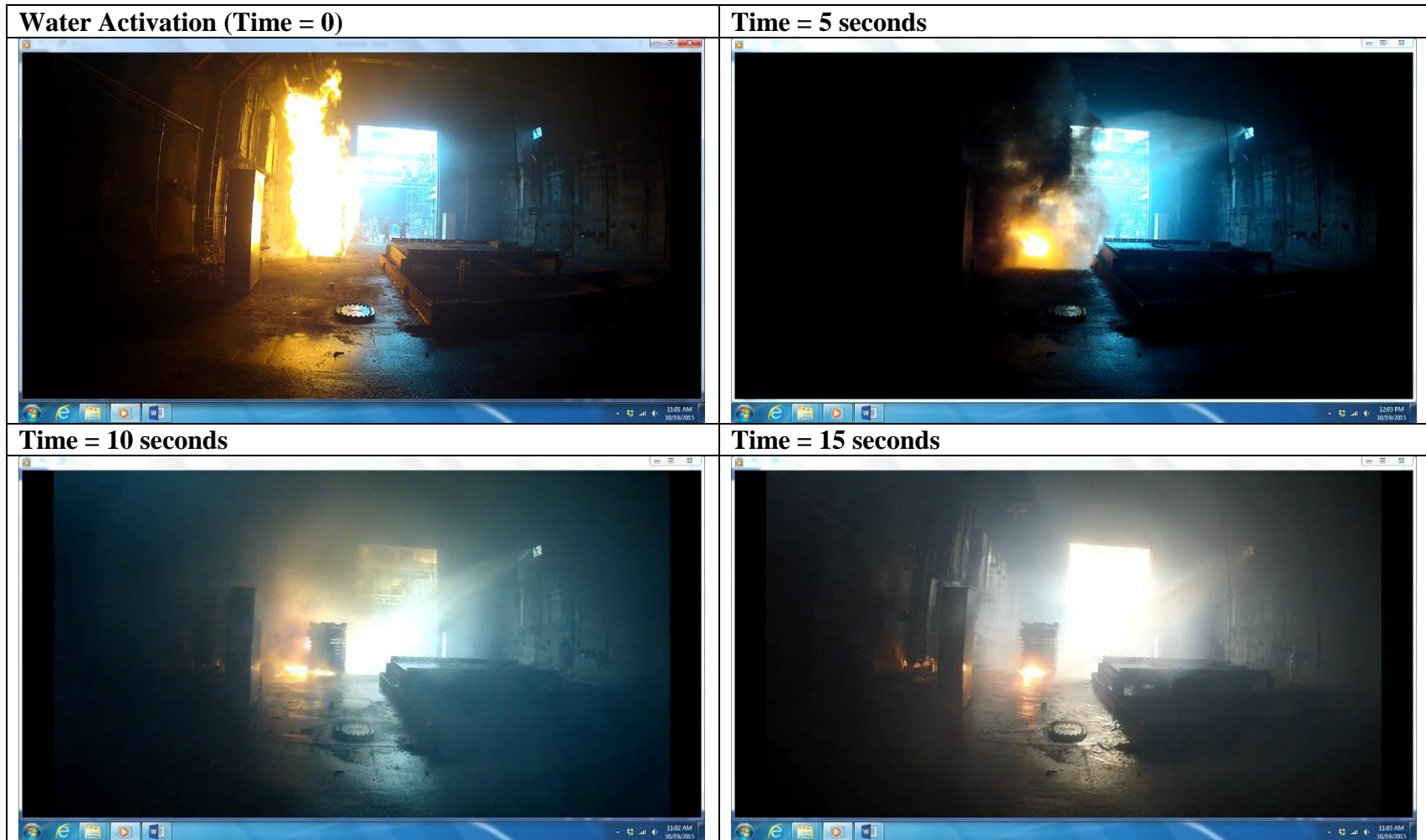
Fig. 24 – Test FS-10 Large Fire Suppression - Delayed Automatic Activation and Targeting
