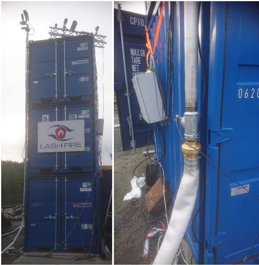
Figure 31. One of the three stacks of 8 ft. steel cargo containers that were used to position the fire monitors above the ground. Each stack consisted of three containers, which resulted in an overall height of 6,7 m. The vertical distance measured from the ground to the inlet of a fire monitor was nominally 7,2 m.
