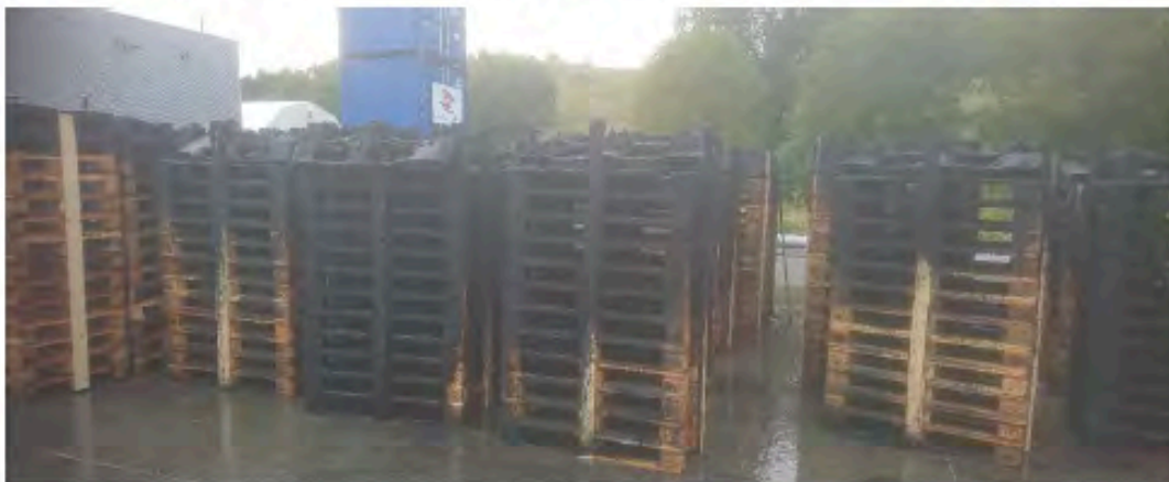
Figure 61. Test 8: The fire damage documented after the test.
