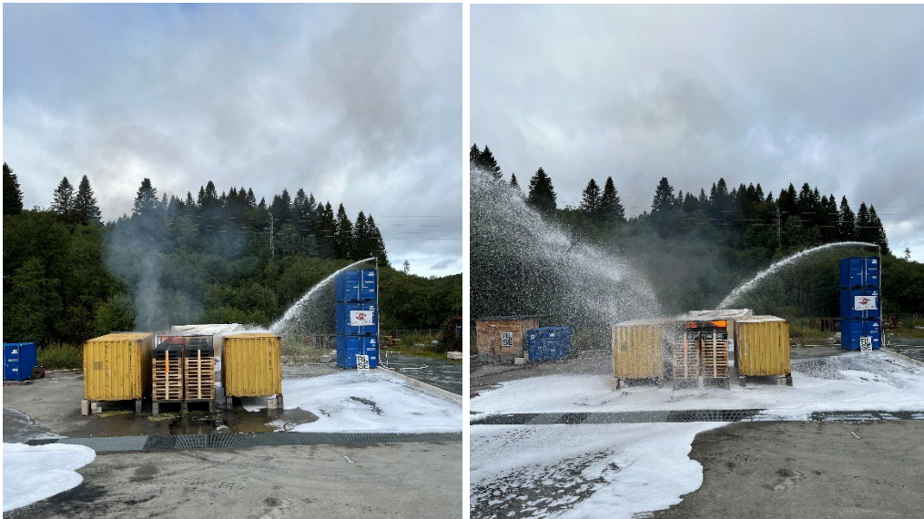
Figure 39. Test 3: The application of CAF from fire monitors A and C, positioned diagonally to each other. It was initially observed that the throw of the fire monitor (C) positioned the furthest from the fire did not reach the fire, but the fire was suppressed by the application of CAF from the fire monitor (A) closest to the fire within a minute, primarily by extinguishing the fire in the ignition tray. After about 02:20 [min:s] from the start of application, the throw of both fire monitors reached the main array.
