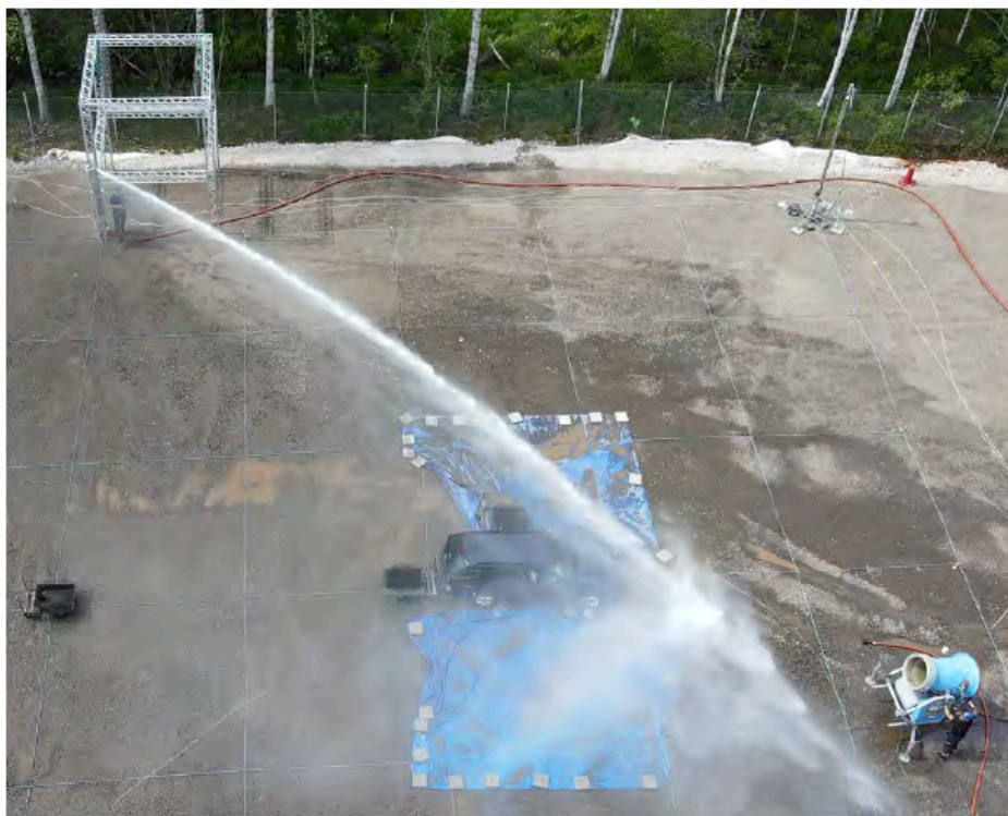
Figure 27. In one test, the snow cannon was positioned near the impact point of the maximum throw length, at an angle of about 45°. Break-up of the solid water stream was observed.
