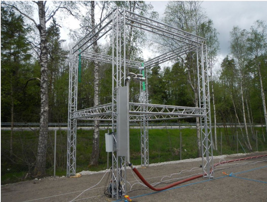
Figure 18. One of the two fire monitors and the truss tower used for the installation. Water was supplied via DN63 fire hoses laid on ground.
