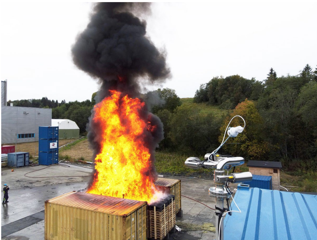
Figure 44. Test 5: The fire size moments before the application of water from fire monitor C, positioned at the South-West corner of the test area, i.e., the fire monitor at the background of the photo. Fire monitor A is observed in the foreground.
