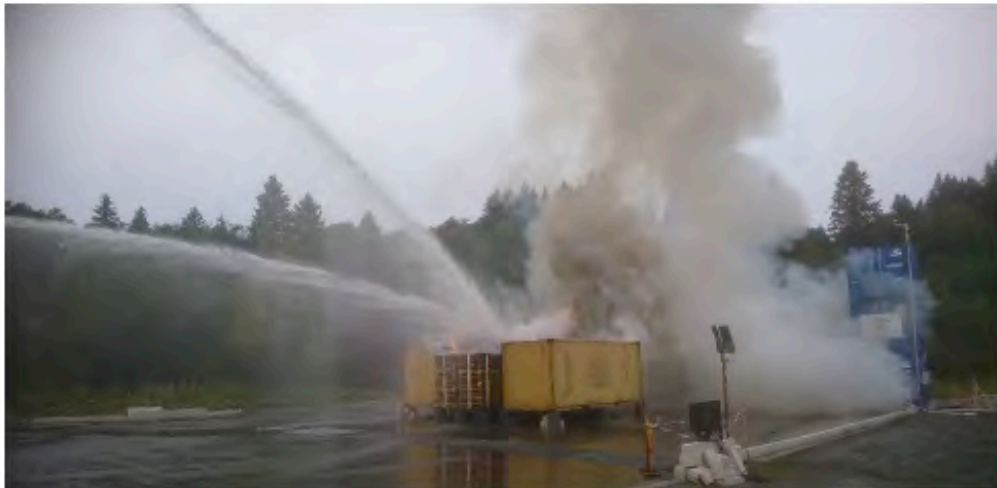
Figure 54. Test 7: Almost immediate fire suppression was observed.
