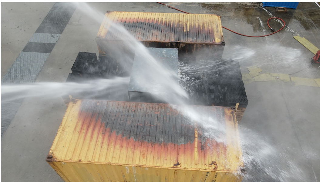
Figure 56. Test 7: A close-up photo of the application of water from fire monitors B and C after fire suppression.
