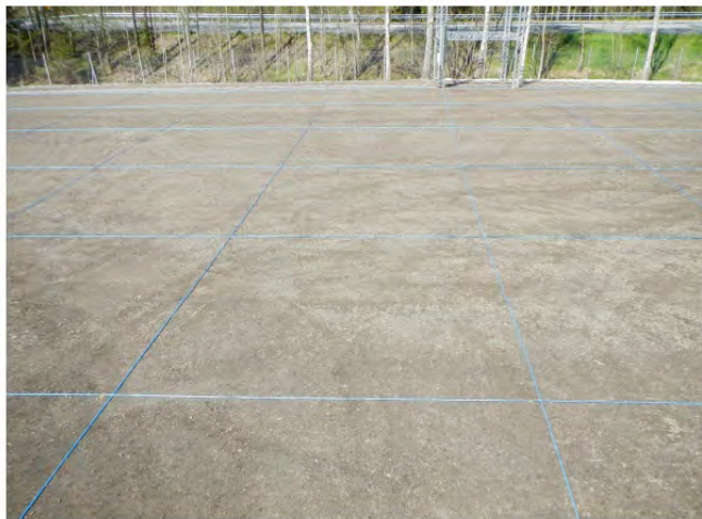
Figure 17. The area was divided into a grid with 5 m x 5 m squares to simplify the positioning of the fire test sources and facilitate documentation of the precision of the water streams from the fire monitors.
