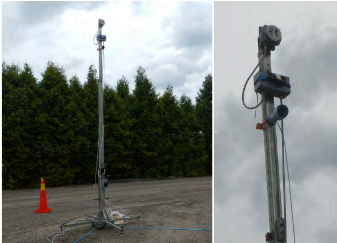
Figure 19. The support for the fire detector. The fire detector was positioned at the top and a video camera was positioned below each detector.
