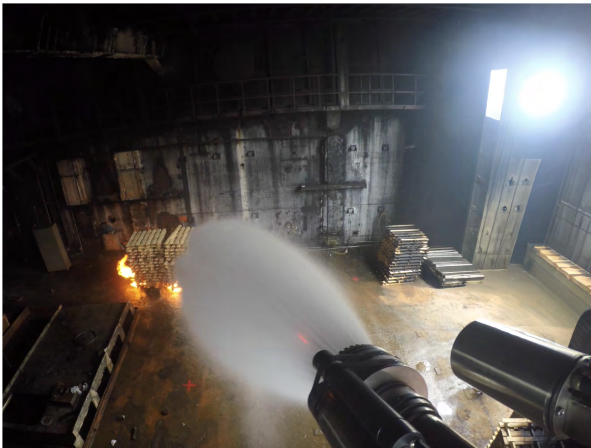
An ARFSS in action during a successful live-fire test conducted by the U.S. Naval Research Labs in collaboration with Jensen Hughes. Credit: Unifire AB.
