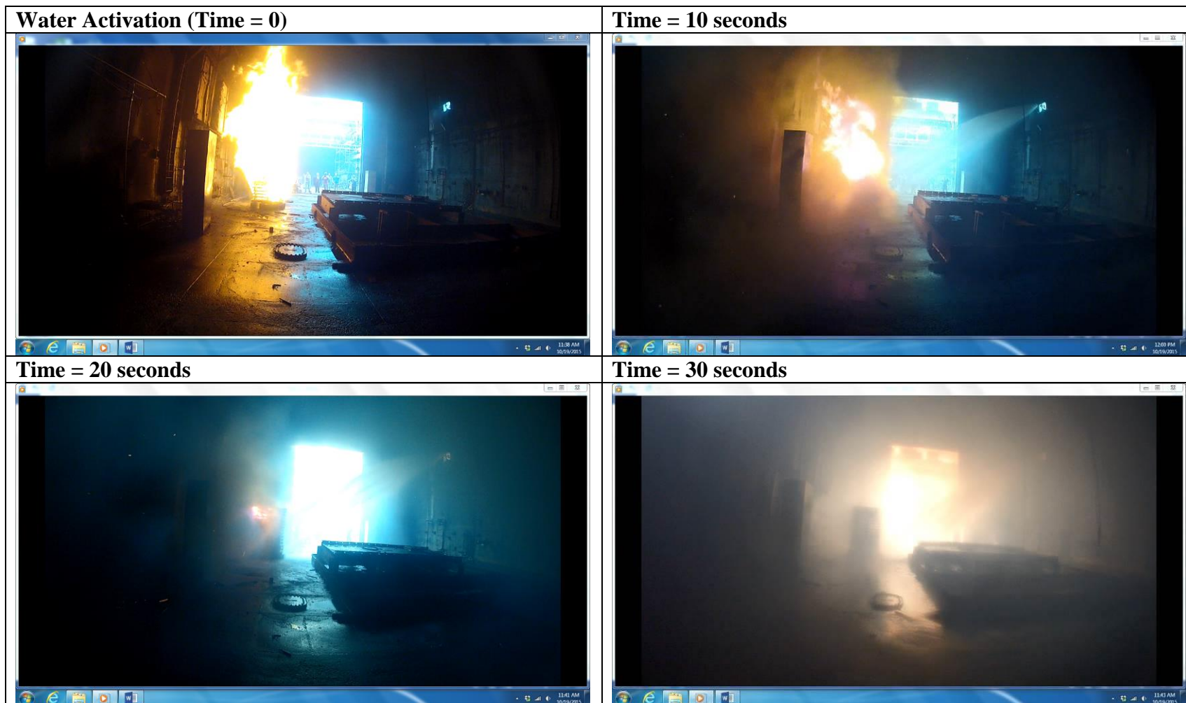
Fig. 22 – Test FS 8 Large Fire Suppression - Pre-programmed Targeting
