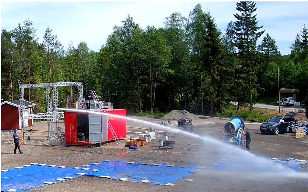
Figure 25. In one test, the snow cannon was perpendicularly positioned near the impact point using a relatively short monitor throw length. Break-up of the water stream was observed, but the reach of solid stream of water was not visually affected by the air velocities.
