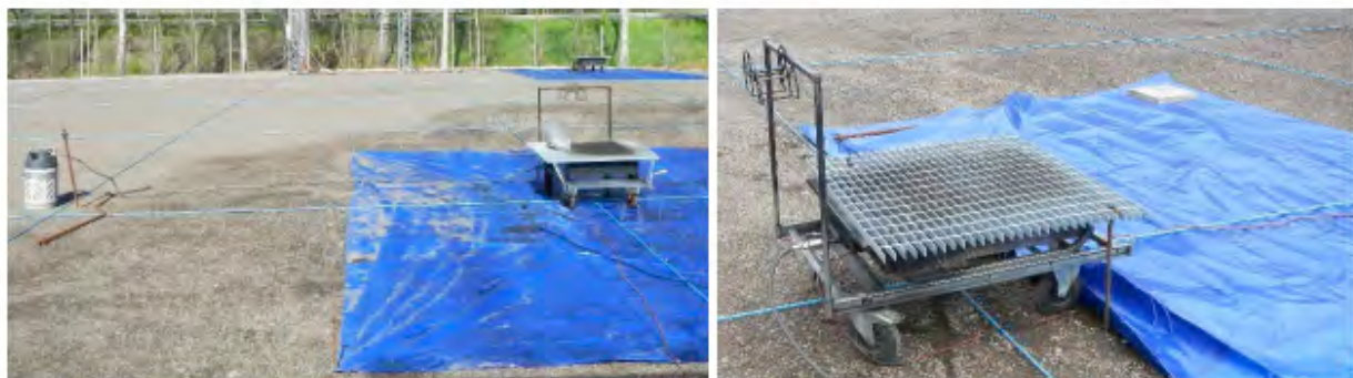
Figure 20. A propane gas burner used as a fire source.
