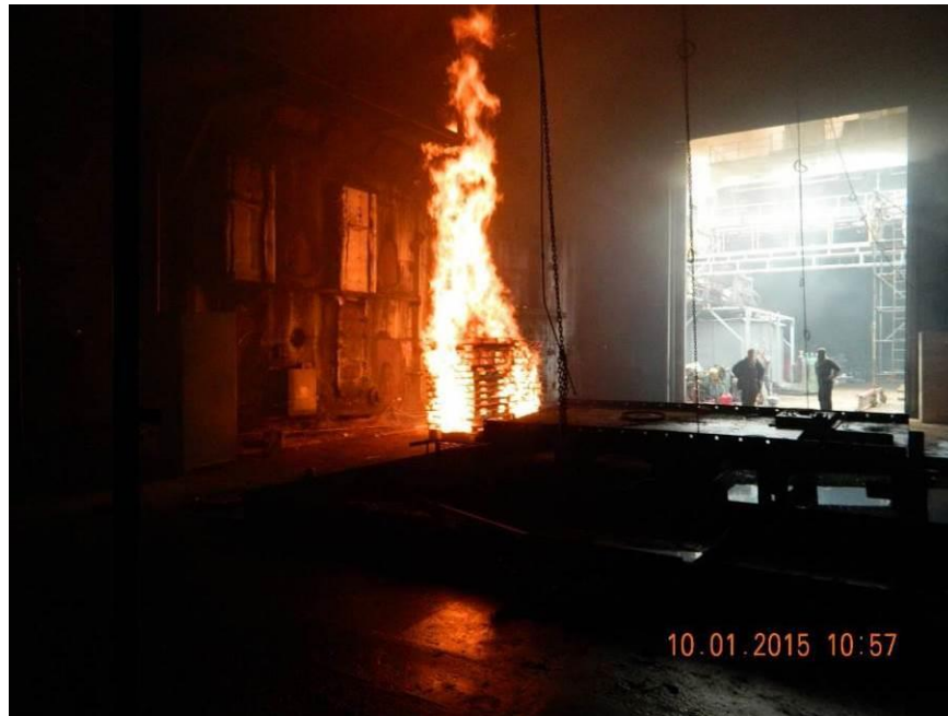
Fig. 16 — Pallet Stack Fire (Full Involvement)
