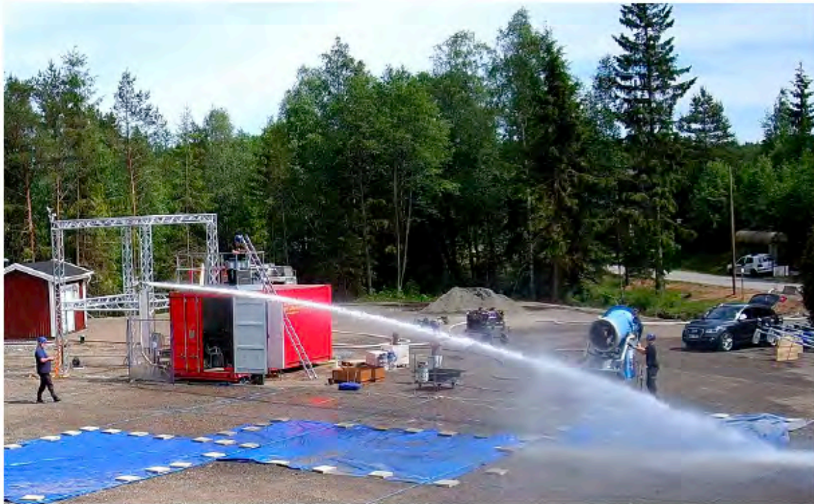
Figure 25. In one test, the snow cannon was perpendicularly positioned near the impact point using a relatively short monitor throw length. Break-up of the water stream was observed, but the reach of solid stream of water was not visually affected by the air velocities.
