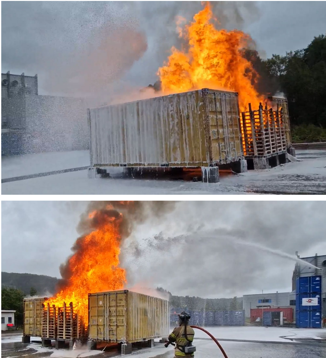
Figure 42. Test 4: The application of CAF from fire monitor C as seen from different viewpoints at approximately the same time. The foam did not reach the seat of fire, which reduced the fire suppression performance.
