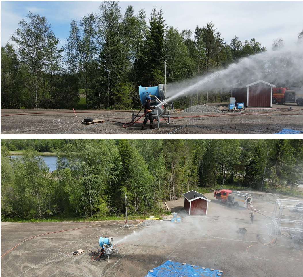
Figure 28. Rain and fog were simulated using a fire hose stream of water directed into the air flow of the snow cannon. The intent was to test the possibilities for fire detection in such environment. Fire detection ability was not influenced.
