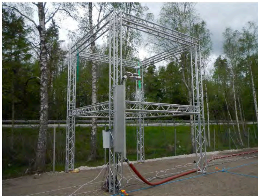
Figure 18. One of the two fire monitors and the truss tower used for the installation. Water was supplied via DN63 fire hoses laid on ground.
