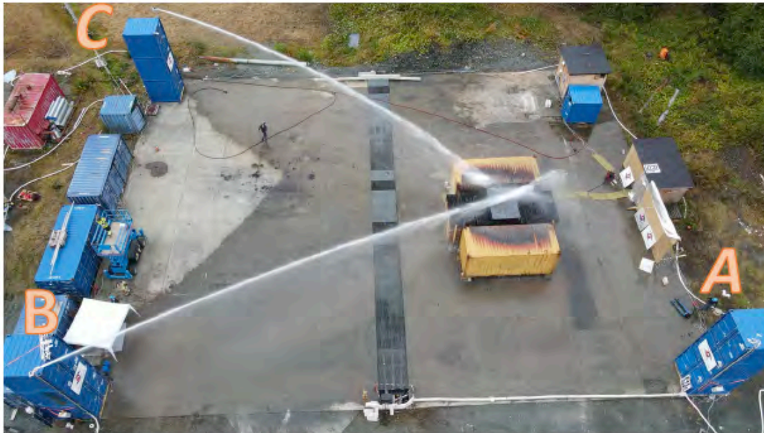
Figure 32. The 40 m (L) by 30 m (W) test area with the positions of the fire monitors (A, B and C) and the fire test scenario set-up.
