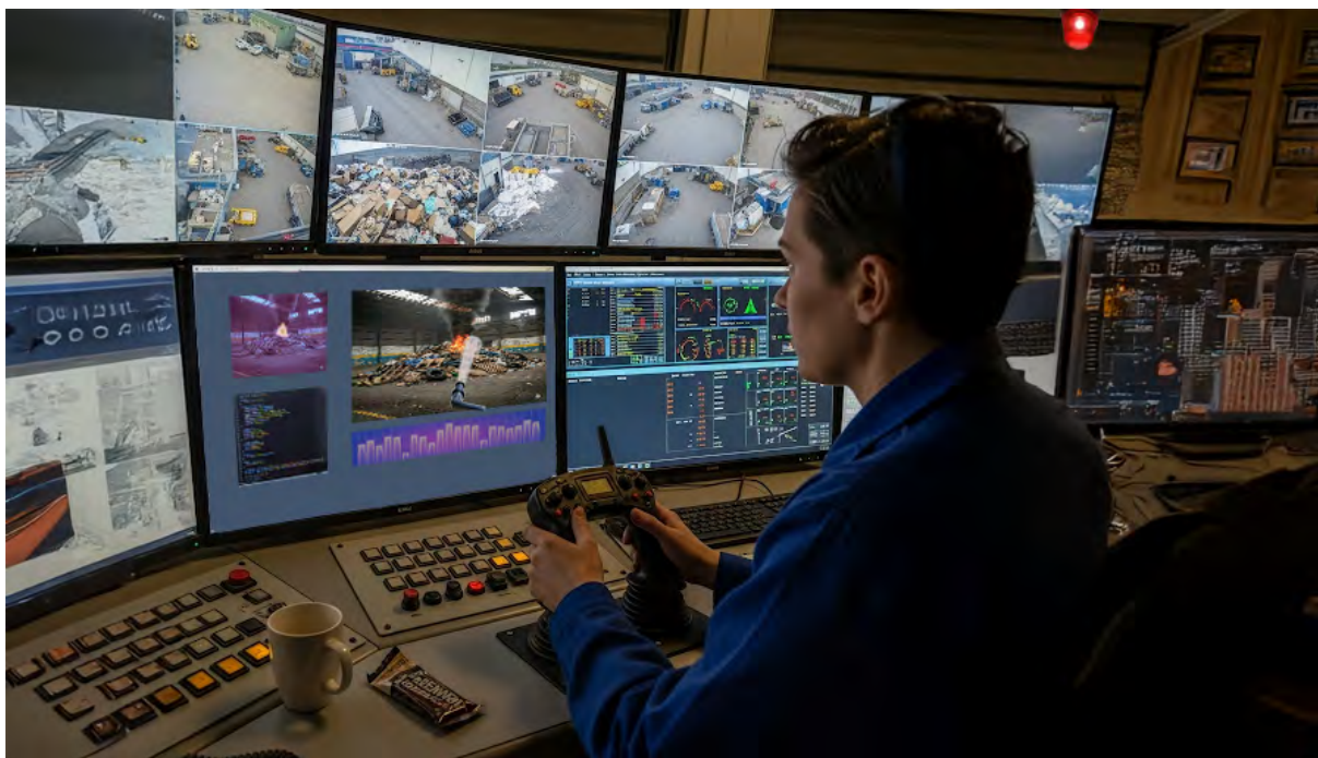
Visualization of a Remote Operator system: detection alerts and live video are transmitted to a centralized command center, where operators remotely aim and discharge fire monitors using joystick controls.
