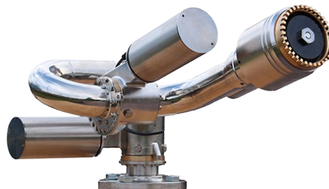
Figure 11. Example of a Unifire FORCE 50 (2") stainless-steel remote-controlled fire monitor with three 24V Brushless DC motors (BLDC) motors and adjustable jet/spray nozzle tip.
