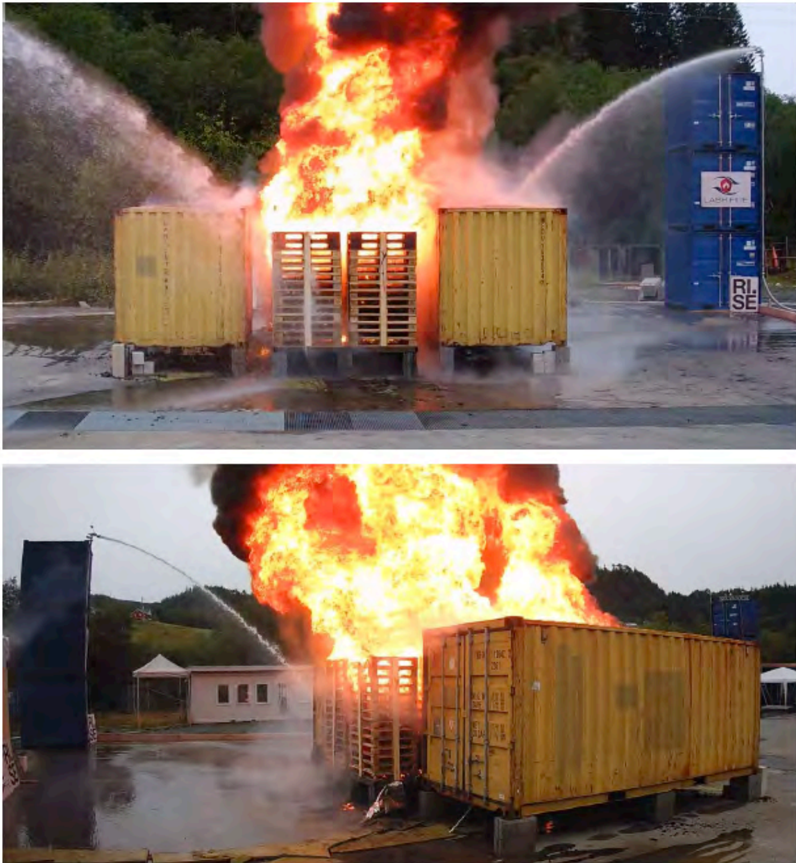
Figure 50. Test 6: The fire size at the start of water application using fire monitors A and C, positioned diagonally to each other, as seen from two different viewpoints.
