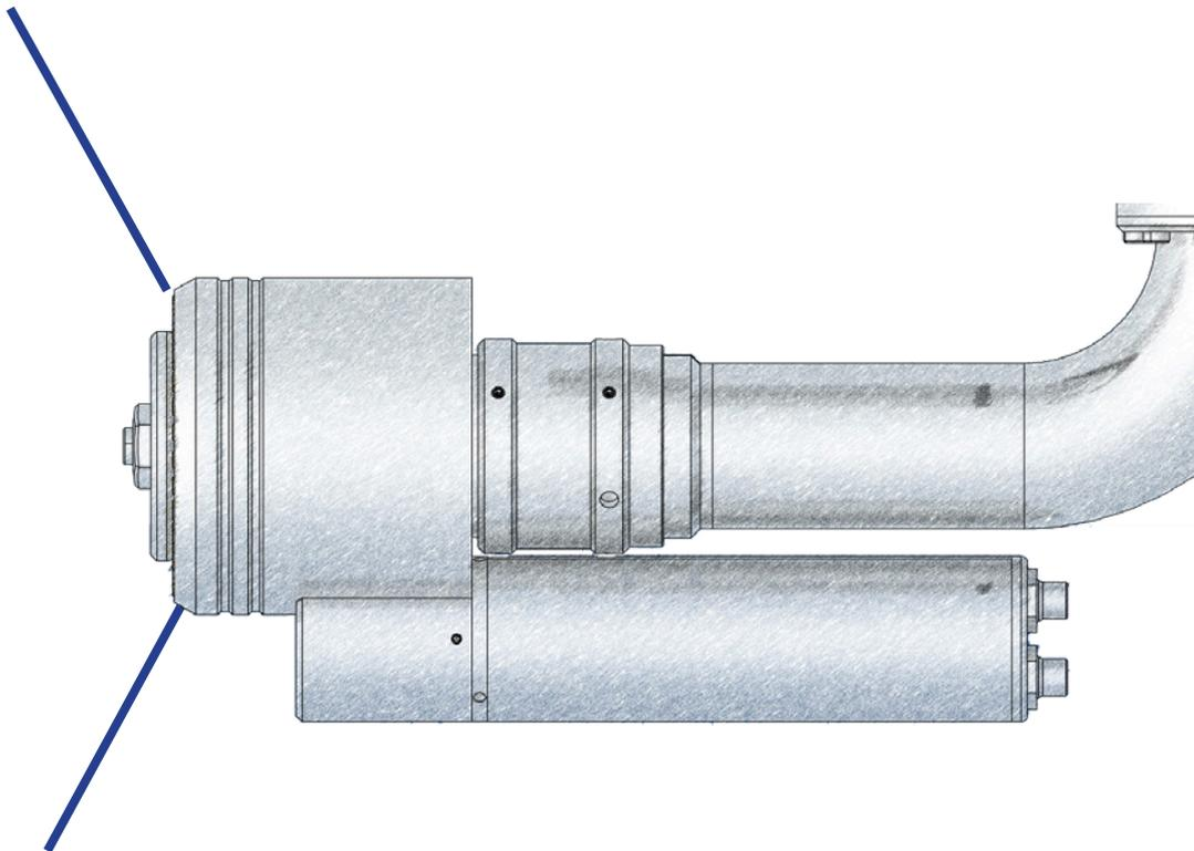
**Set the nozzle minimum (Motor 6), to stop just before the mechanical stop.**
