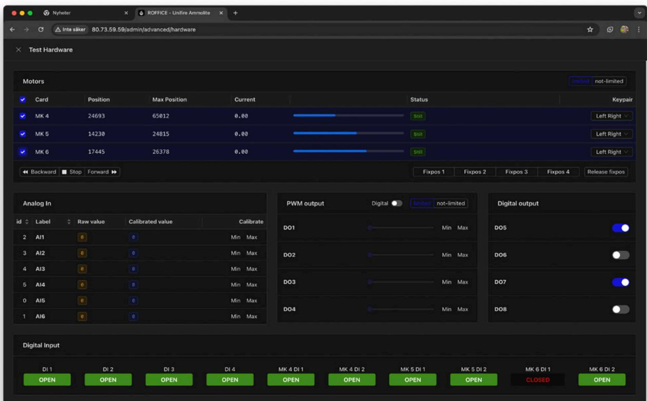
8) This opens up the system overview page. Here, you can read the position of the motors, calibrated max, see the actual real time current draw (A), and the motor status. You can also see the status of the generic digital and analog inputs and outputs. (MK4 is usually horizontal, MK5 usually vertical, and MK6 usually nozzle jet/spray.)
