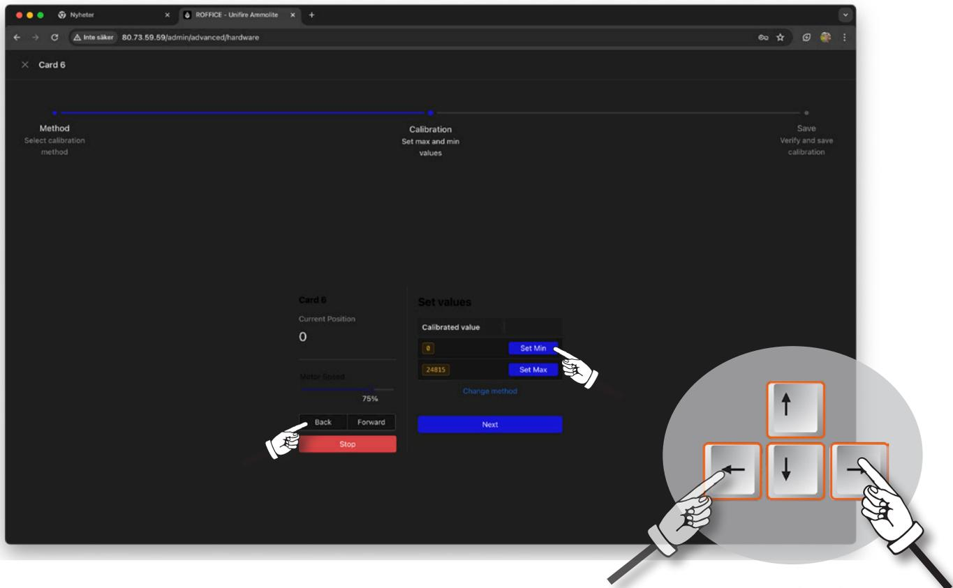
23) Run the motor to the Min (minimum) position, which is fully retracted and provides the widest spray angle). Click Set Min.
