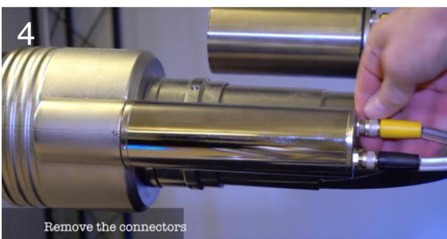
To inspect the nozzle motor, first remove the connectors.
