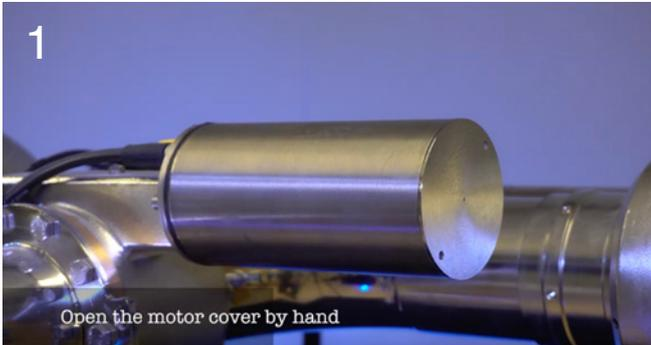
Open the motor cover for the vertical motor.
