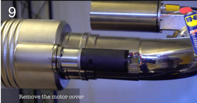
Wipe off any moisture, inspect, and cover the motor with some WD40 before reassembly.
