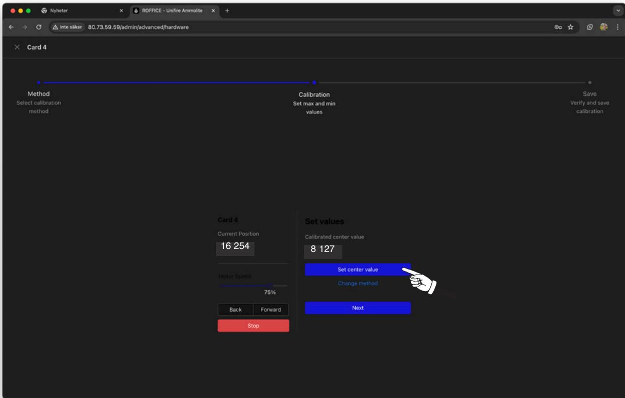
13) **Example 1, Center Method:** When you have moved the robotic nozzle to the required center position, click “Set center value”. (Typically, the calibrated total range will be exactly twice the calibrated center value.)
