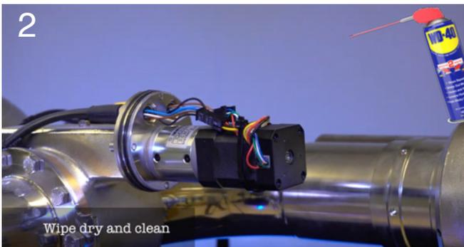
Wipe off any moisture, visually inspect, and then cover the motor with some WD40 before reassembly.
