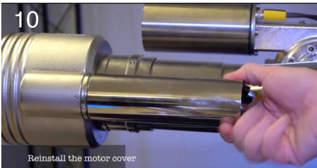
Reinstall the motor cover by hand.
