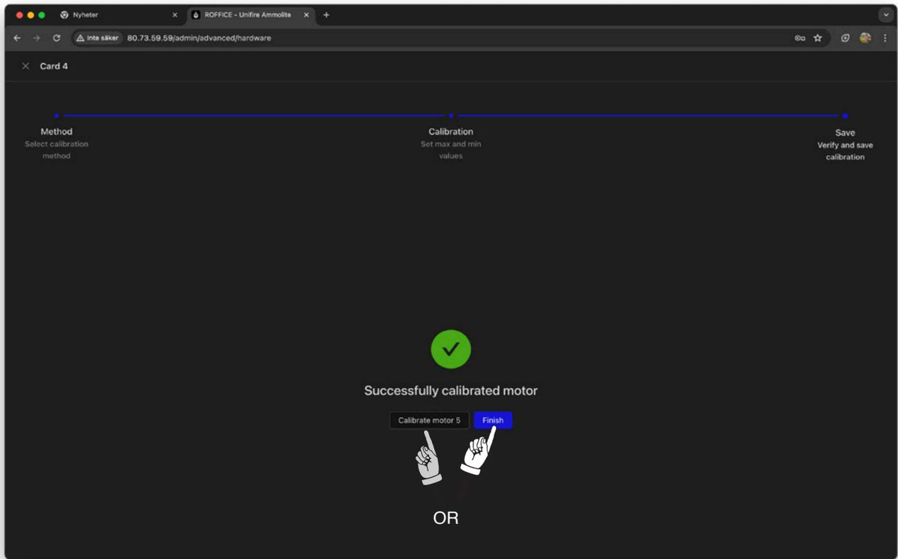
15) When you have successfully calibrated motor 4, you may want to continue with motor 5 (and repeat steps 12-14), or exit calibration. (Be sure that all connected motors are calibrated prior to operating the system.)
