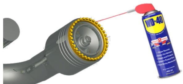
Wiping off and putting a few drops of DW40 on the stream shaper prevents the build up of grime and goo. Please perform when required.
