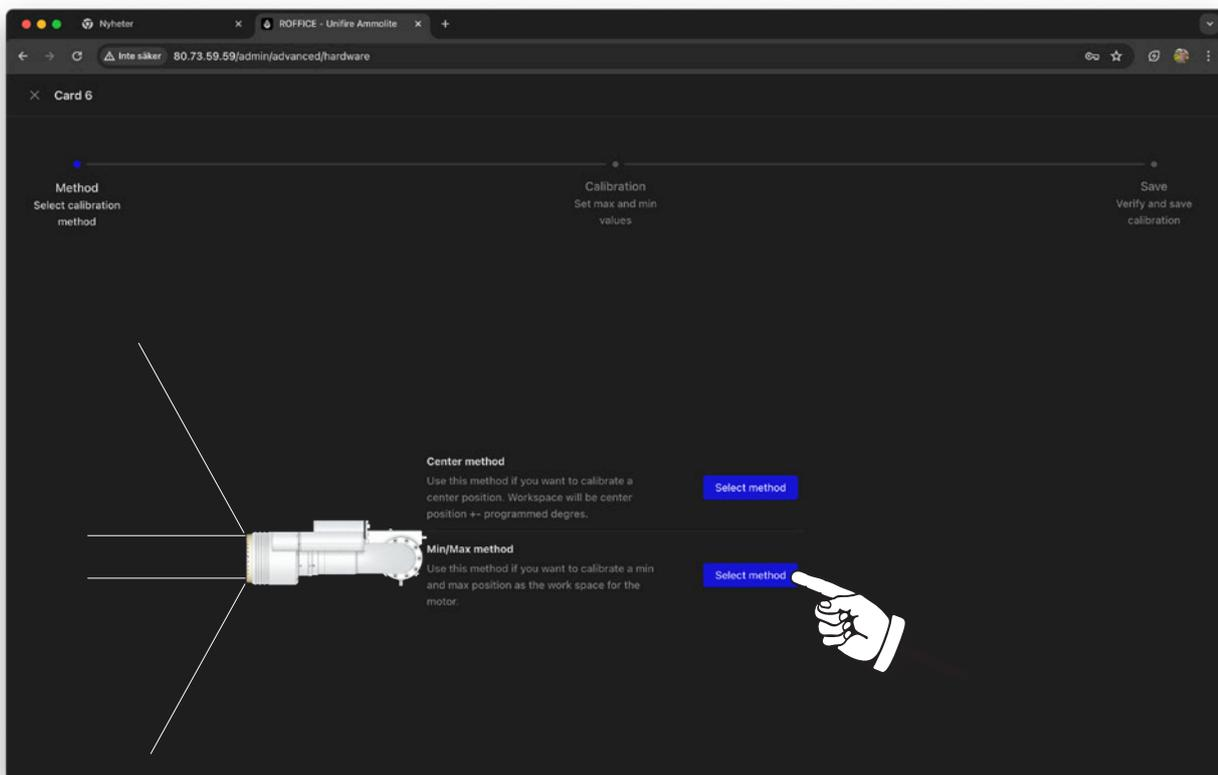
22) The INTEG nozzle motor is always calibrated using the Min/Max method (not the Center method).
