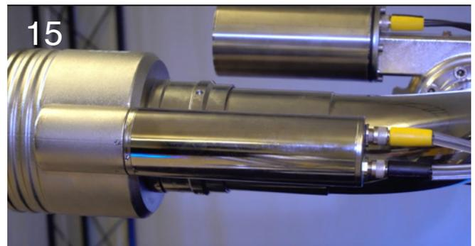
Install the connectors. Make sure to tighten the M12 connector by hand (do not use any tools).
