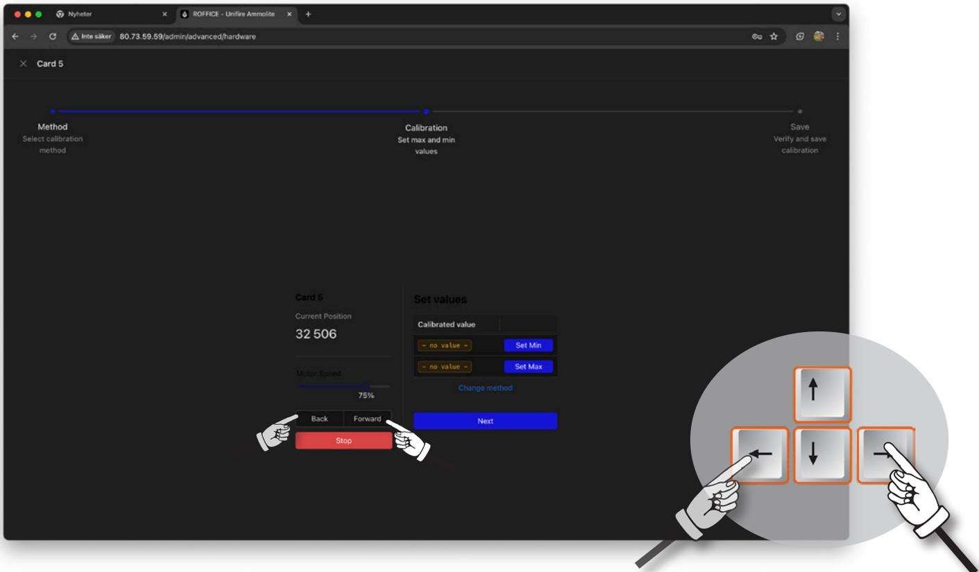
17) To run the motors please use the Back or Forward buttons - or use the Arrow keys on your computer. Move the robotic nozzle to the required minimum position.
