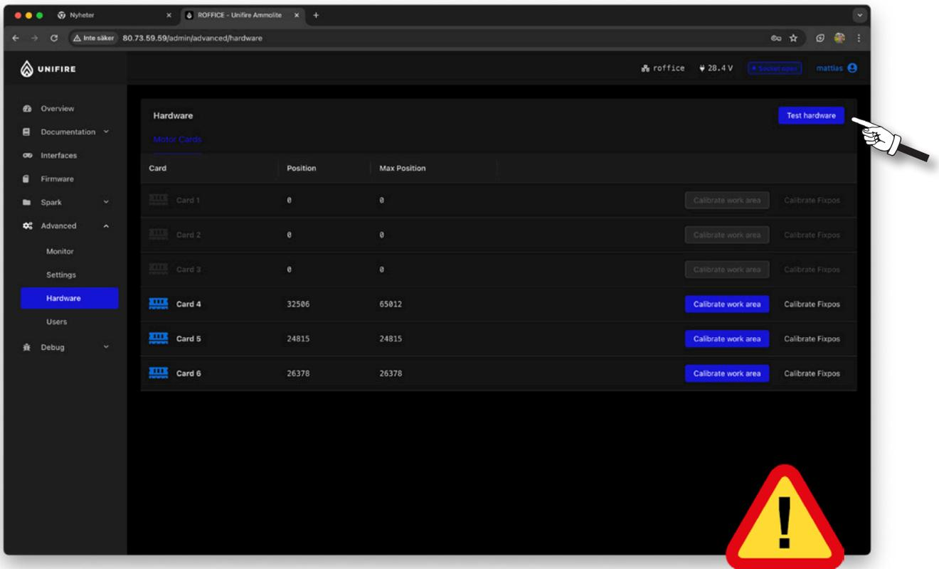
24) Next you can test the motors and the calibrated range directly from your PC. From the Hardware tab, please click Test Hardware. **Please note that “Test Hardware” blocks any other Joystick or controller connected to the system. Hence, you must remember to exit this view when done.** ⚠
