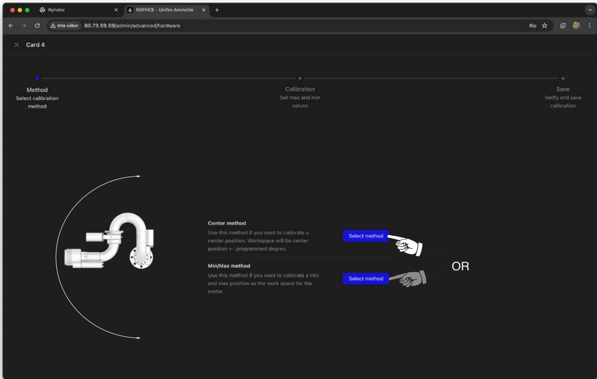
11) Now choose Center method or Min/Max method. Center method is used for special applications when the operating range is preset in the software - typically to  $\pm 90^\circ$  exactly. Min/Max allows you to set the end positions freely. In Example 1 (steps 13-15, below), we use the Center method; in Example 2 (steps 16-20), the MIN/MAX method.
