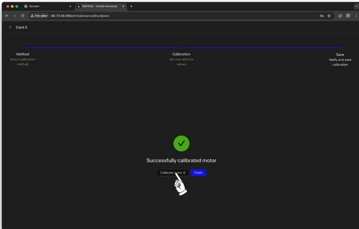
21) **INTEG Nozzle Tip Calibration:** Next, calibrate the INTEG jet/spray nozzle motor (typically, motor 6).
