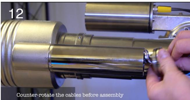
Counter-rotate the wires at the end of the end-cap 720° before assembly.
