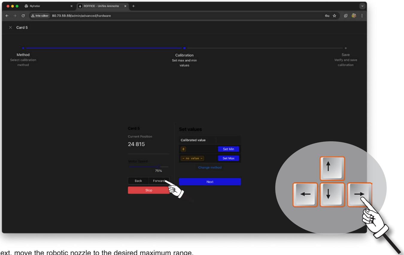
19) Next, move the robotic nozzle to the desired maximum range.
