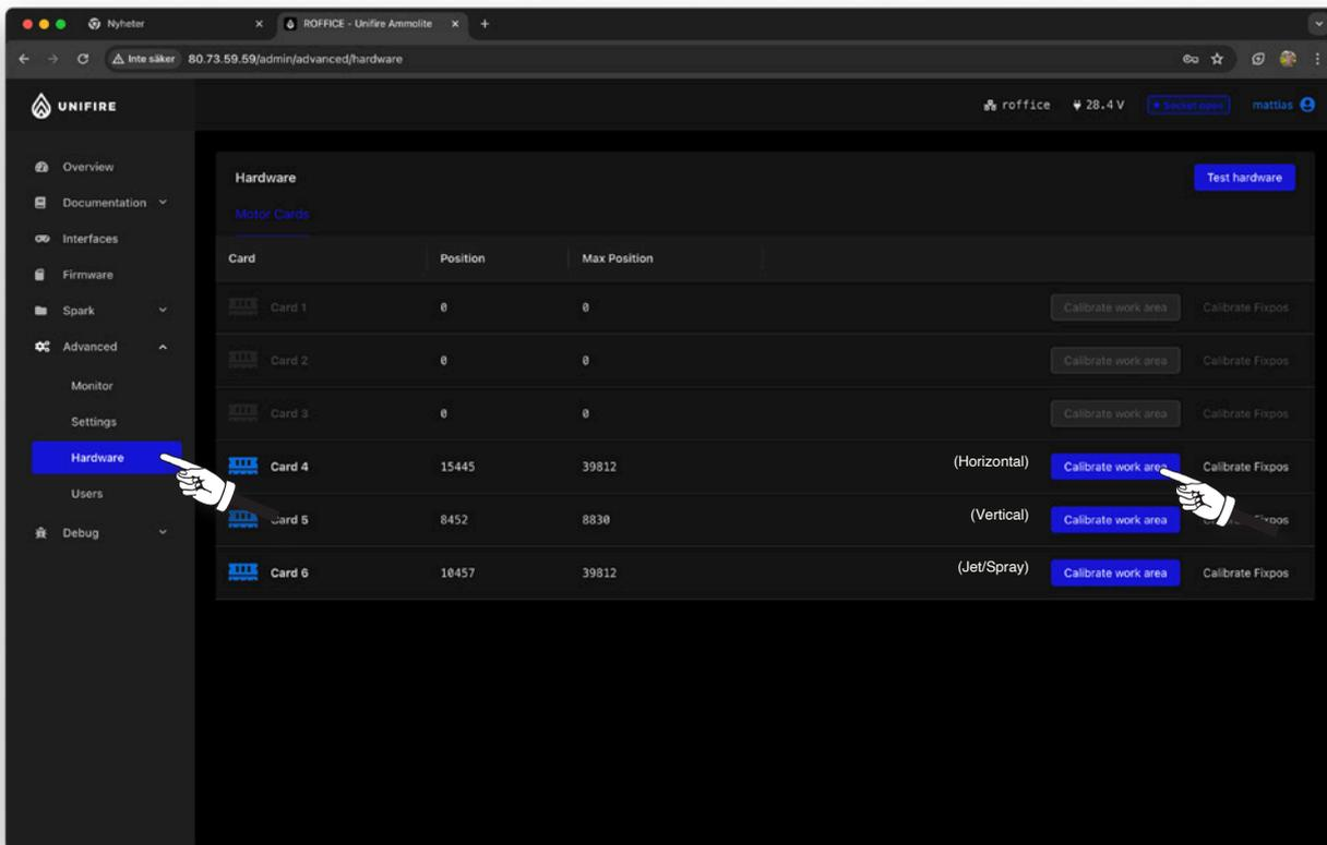
10) ....and then Hardware..., and then select a BLDC motor driver to calibrate. In this example, we start with Card 4, the horizontal motor with normal orientation.
