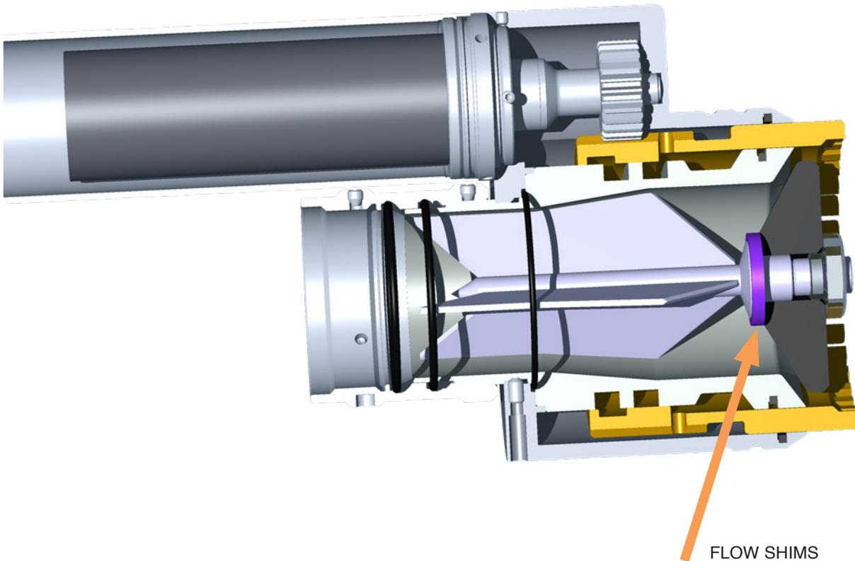
Flow shims are 3D printed specifically to order.
