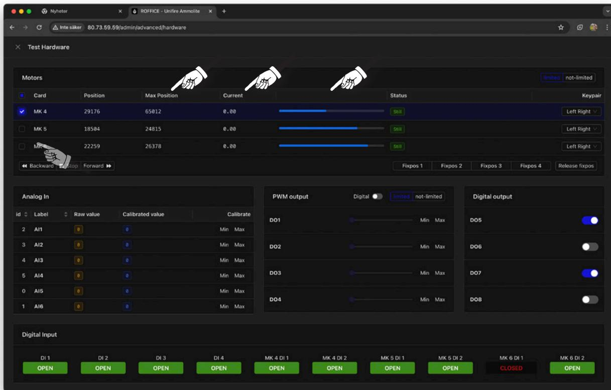
25) When you run the motors, you can read the absolute position on pulse-level, and you can see the real time current draw for each motor. The blue bars show the current real time position in relation to the calibrated range.
